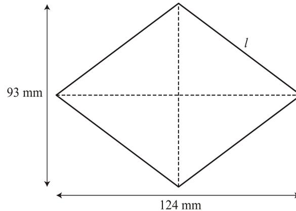
$$l^2 = \left(\frac{d}{2}\right)^2 + \left(\frac{D}{2}\right)^2 \rightarrow l^2 = 46,5^2 + 62^2 \rightarrow l = \sqrt{6006,25} \rightarrow l = 77,5 \text{ mm}$$
